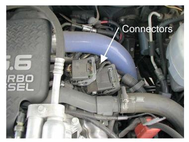
Notice: Use caution when inserting connector bodies. If the connector does not slide smoothly, remove the connector, inspect the pins, and retry installation.
